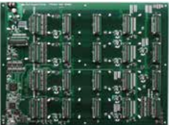
Example of a custom burn-in board
