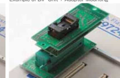
Example of DIP Unit + Adapter Mounting
