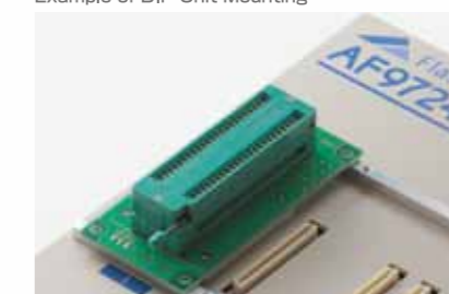
Example of DIP Unit Mounting
